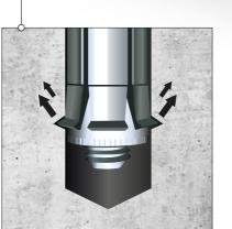
**Heavy Duty Self-Undercutting Anchors** create a durable mechanical interlock with flooring, giving exceptional pull-out resistance under extreme
