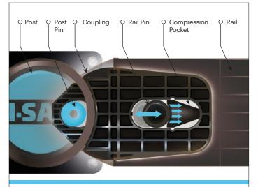
**PHASE 1:** Memaplex<sup>™</sup> rail flexes to absorb impact, initiating the rail pin to slide forward and transfer load energy to the compression pocket.
