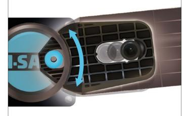
**PHASE 2:** Compression of the pocket continues to disperse energy as the coupling rotates around the post pin to activate further absorption.
