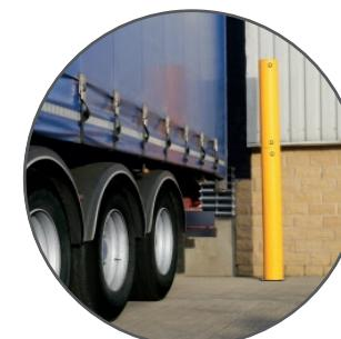
Higher level bollards give a strong visual alert for reversing HGV drivers, preventing costly damage to service yard infrastructure.
